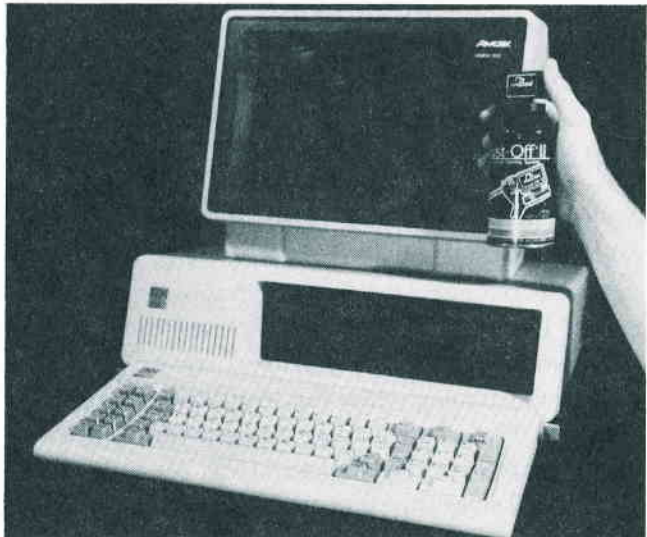
Fig. 5-3. An antistatic spray for computer equipment. (Falcon Safety Products, Inc., Mountainside, New Jersey)
