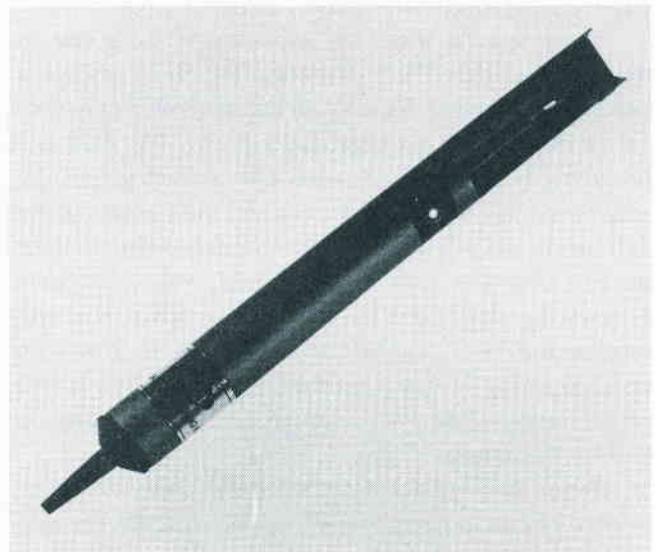
Fig. 6-24. The spring-driven plunger in the solder vacuum pump is used to pull hot solder off a connection.
