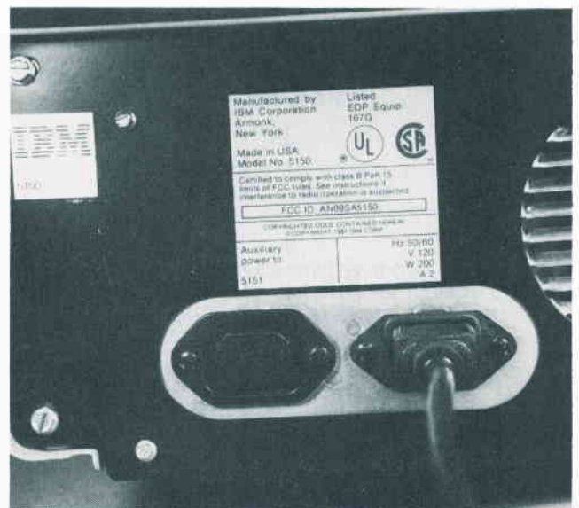
Fig. 2-38. A special connector provides power to the IBM monochrome display unit.
