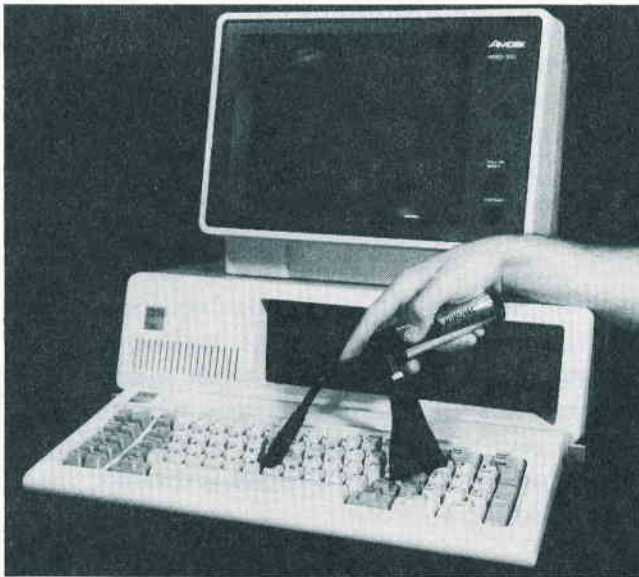
Fig. 5-4. A handy tool for cleaning dust off keyboards and circuit components. (Mini-Vac, Inc., Glendale, California)
